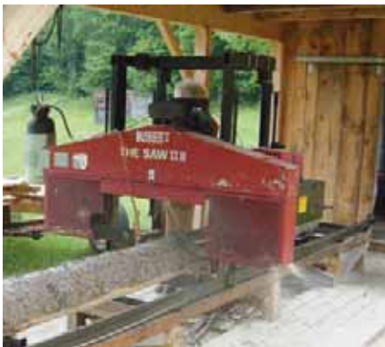
The mill is designed for the operator to walk backwards, as he pulls along the saw carriage.
