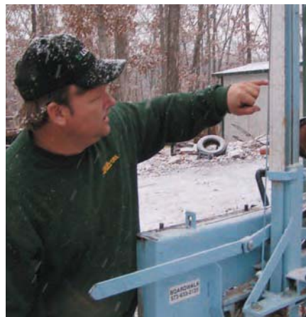
The height gauge has scales for common lumber thicknesses, and accounts for the kerf of the blade.
