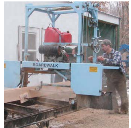
John Arnett pushes the blade through a stack of 3/4 oak to prepare it for the moulding machine inside the shop.
