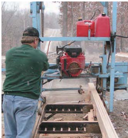
The Arnett brother’s mill does double duty as Ron uses it as a straight line rip saw. Although not the ideal tool for the job, he says that it is accurate enough for their molding.
