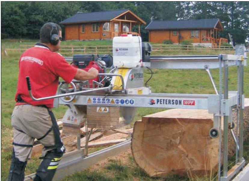
The *original* commercial portable swingblade mill -
