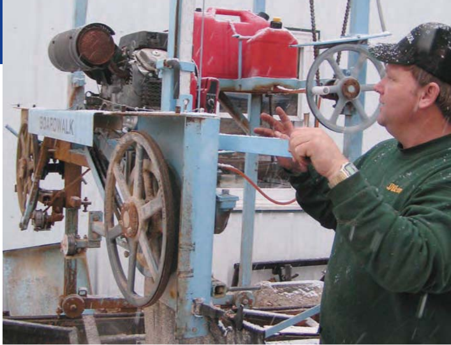
The lever to engage the band wheels slides the engine on its mount to tighten the drive belts. The guards were removed for demonstration only, and were replaced before the engine was started.
