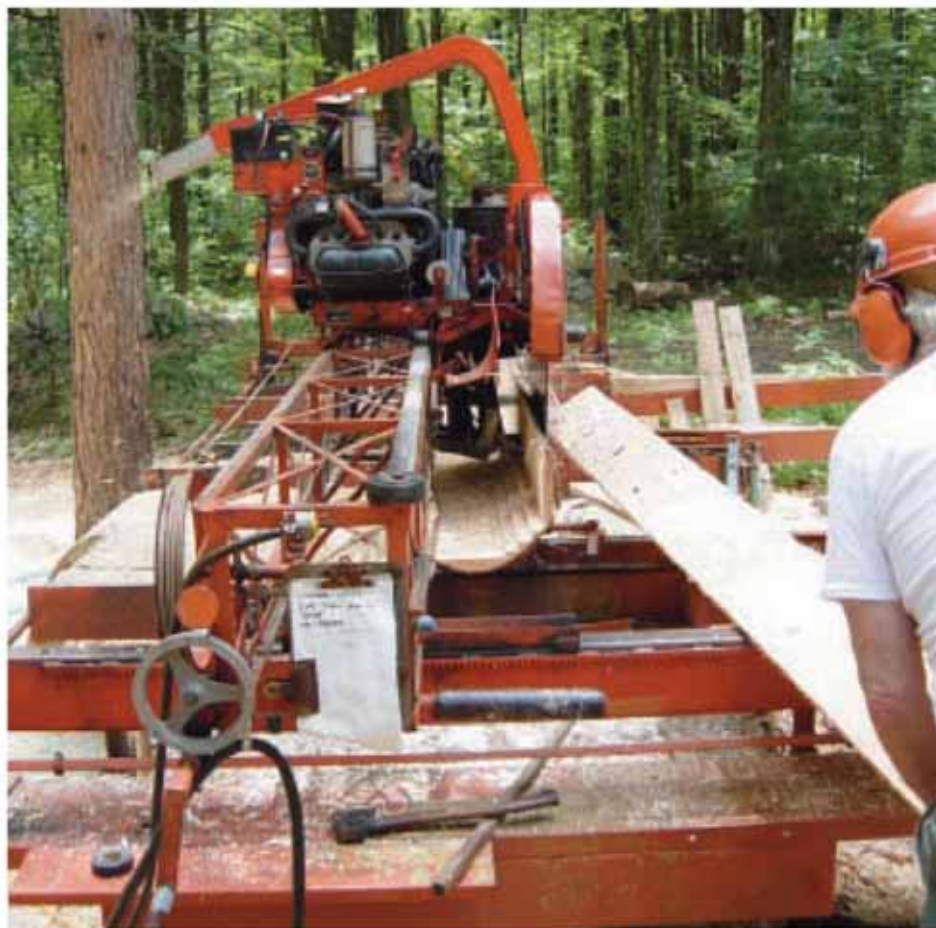
As the saws are making the next cut, Rex removes a board that has just been sawn and returned by the carriage to Rex at the operator's position.
