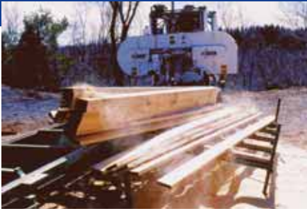
Production from the entire log is being dumped simultaneously onto the lumber deck after being sawn.
