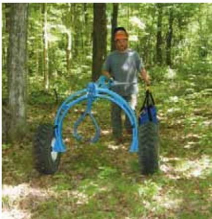
With the tow tongue removed, the fetching arch may be wheeled directly to where a log is to be removed.
