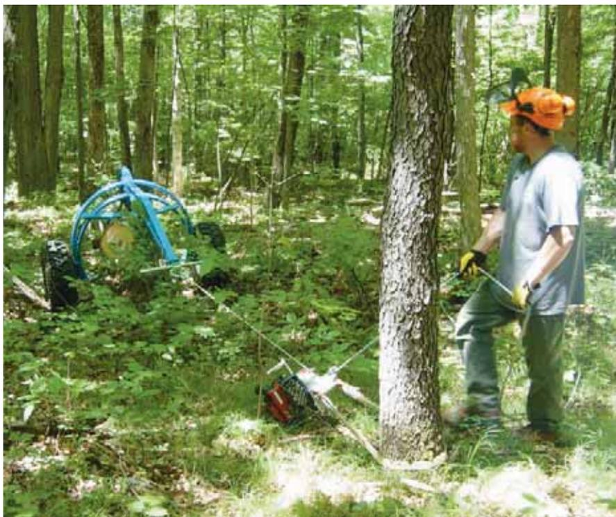
It is possible to skid a log up-slope with a portable winch and the arch.
