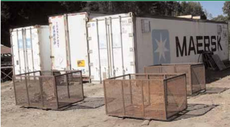
Metal kiln baskets waiting in front of the two kiln boxes, one on each side of the storage box.
