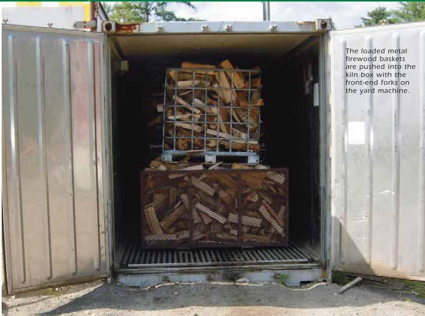
The loaded metal firewood baskets are pushed into the kiln box with the front-end forks on the yard machine.
