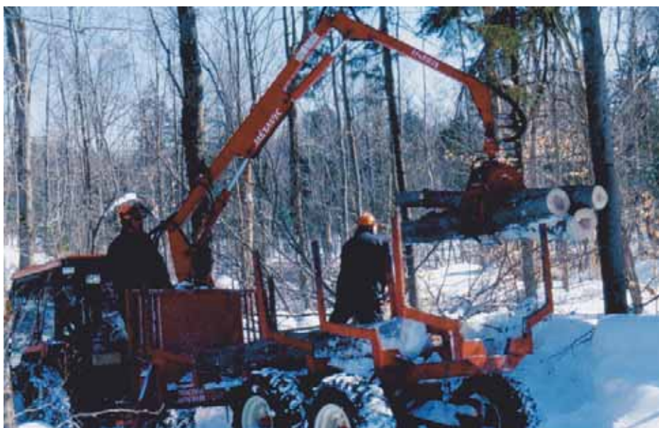
Jean Claude employs forwarding units consisting of a rugged wheel tractor combined with trailer and loader.
