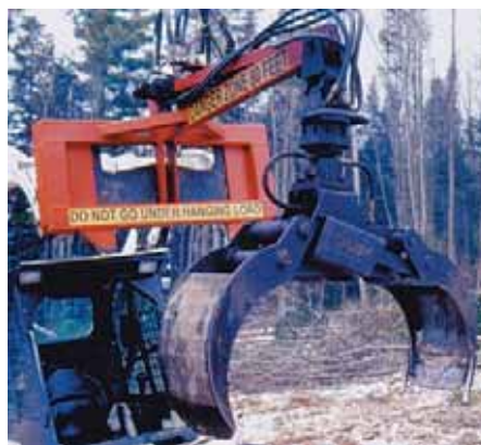
The skid-steer grapple is designed to be suspended from a high position on the frame at the front of the machine.
