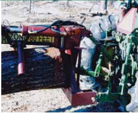
This close-up of the 3-point hitch shows the weight of the grapple attached in a low position.
