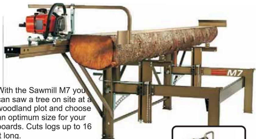
With the Sawmill M7 you can saw a tree on site at a woodland plot and choose an optimum size for your boards. Cuts logs up to 16 ft long.
