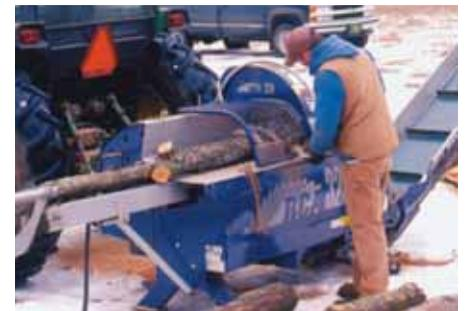
*The Tajfun processor fastens to the 3-point linkage system of the tractor. 30 hp is the stated minimum power required.*
