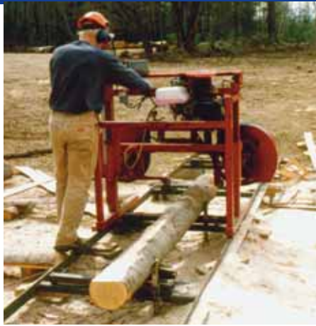
Gouge producing construction lumber from small logs cut on property.
