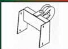
Top pulley for high spooling point on 3001, 4001, 5001.
