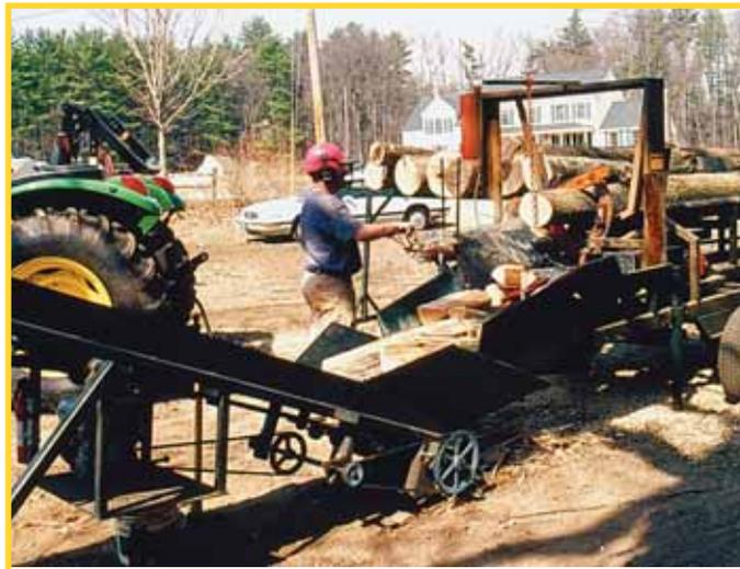
Deere tractor. The Built-Rite firewood processors are hydraulically operated, and with the PTO models one has the choice of hooking the processor hoses onto the tractor's hydraulic pump or using a separate "slide-on" pump, which fits over the tractor's PTO shaft. Steve chose the latter.
