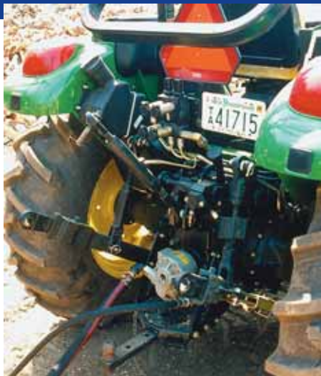
Most operators prefer the slide-on pump because it eliminates the task of attaching and removing the hoses each time it is used.
