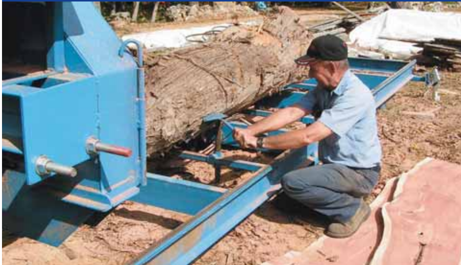
Log clamps are a pair of adjustable cams on handles. Note the two large nuts on the side of the mill for adjusting blade tension and tracking.
