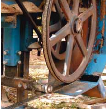
The blade guides are sealed bearings above and behind the blade, and a brass plate below it.
