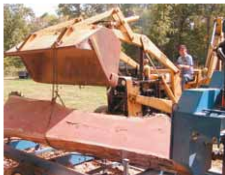
Floyd’s “hydraulic log turner” is his backhoe loader. He only uses it on logs that are too heavy to turn with a cant hook.
