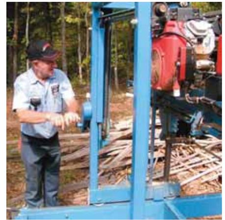
*Adjusting the blade height. As with most manual mills, Mister Sawmill uses a crank to adjust the height. A ratchet holds it in place.*
