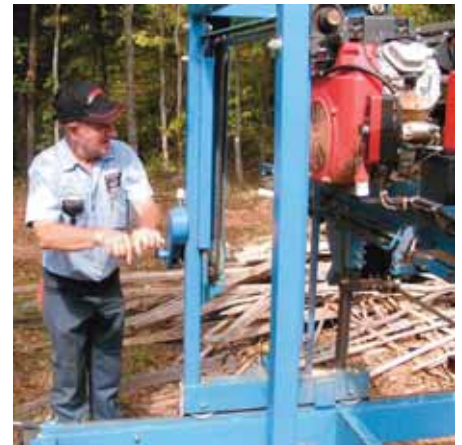
Adjusting the blade height. As with most manual mills, Mister Sawmill uses a crank to adjust the height. A ratchet holds it in place.
