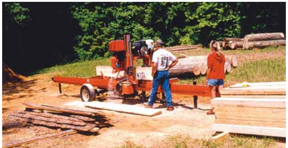
Fred decided to include the log deck package – a manually operated winch, a manually operated log turner, and a toeboard.
