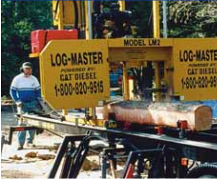
The 26-hp motor and 30-in.-diameter band wheels can handle logs up to 36 in. in diameter and 24 ft. long.
