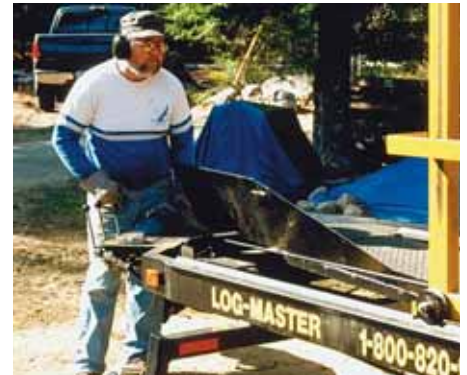
Mike likes the remote operator station that eliminates the need to walk the length of the sawmill with each saw cut.
