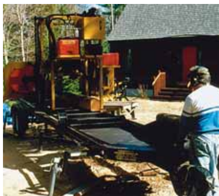
The mill's bed frame is constructed of 3-in. x 6-in. tubular steel, 1/4 in. thick.
