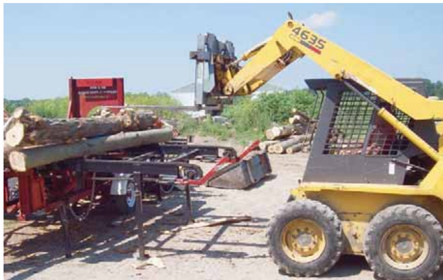
Pete's handicap requires a live log deck to feed the processor. His nephew operates the loader.
