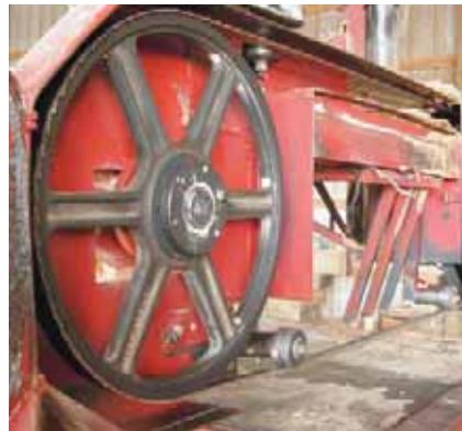
Keener Built behind the cover. Note that the backing bearing is at the top of the blade.
