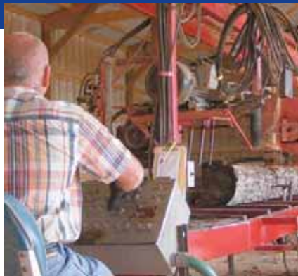
Opening cut on a black oak log. Note that the track and hydraulic hoses are above the log deck where they are less likely to be damaged. This design also eliminates posts that must clear the log.
