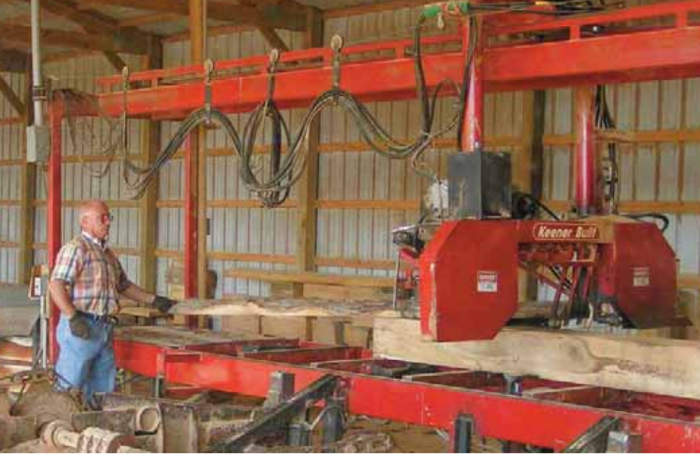
David Douthit uses the drag back to pull a slab off the log. Heavy slab cuts like this one will go to the resaw to be cut into stakes.
