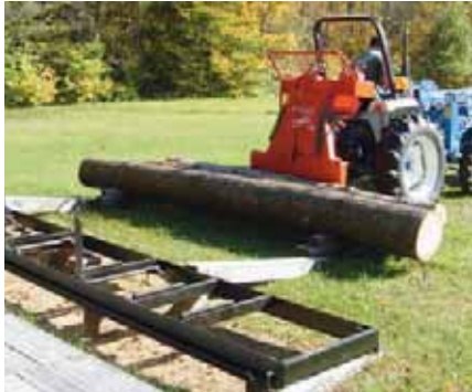
The blade of the winch is used to nudge the log along the ground-level log deck at the sawmill.
