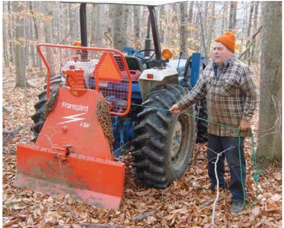
Albert Wood uses the rope control for safe operation.
