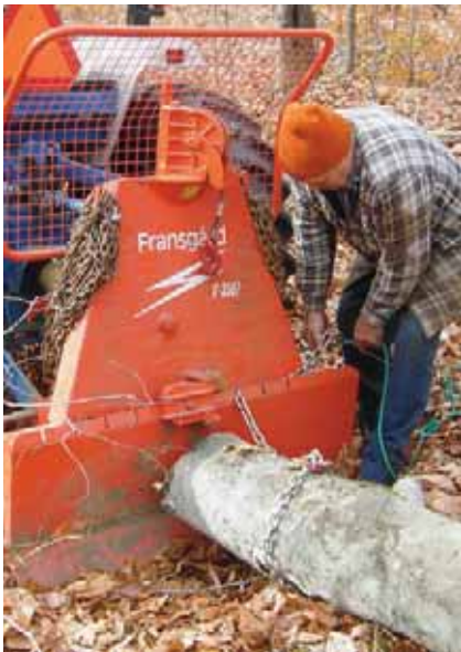
The log is chained to a notch on the draw bar of the winch.
