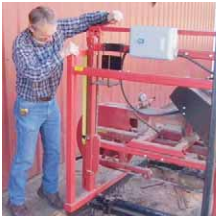
The hand crank adjustment uses acme thread rods on both sides of the head rig and is geared for five revolutions per inch travel.
