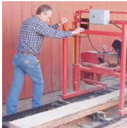
Pushing the blade through the wood requires only light pressure if the blade is sharp. The 7.5-hp, single-phase motor is the usual power source for this mill.
