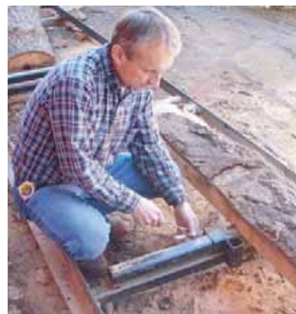
Using the spring-loaded clamp to hold the cant, the cleats are low enough to allow a final minimum cut thickness of 1 inch.
