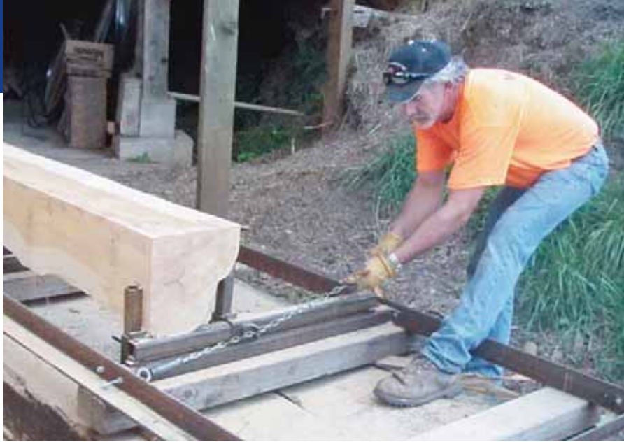
Shawn sets the clamp. He says that the spring-loaded clamping system does a good job holding even the larger logs in place.
