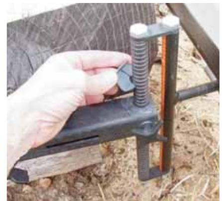
Adjusting the height of the cut. The bracket allows 12 inches of vertical travel. The slots allow movement in 1/4-inch increments, and must be adjusted on both ends after each cut.
