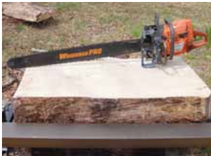
The Big Mill Basic setup, ready to start cutting. The Husqvarna 372 is a little on the small size, but managed to cut the catalpa log with no problem.
