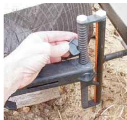
Adjusting the height of the cut. The bracket allows 12 inches of vertical travel. The slots allow movement in 1/4-inch increments, and must be adjusted on both ends after each cut.
