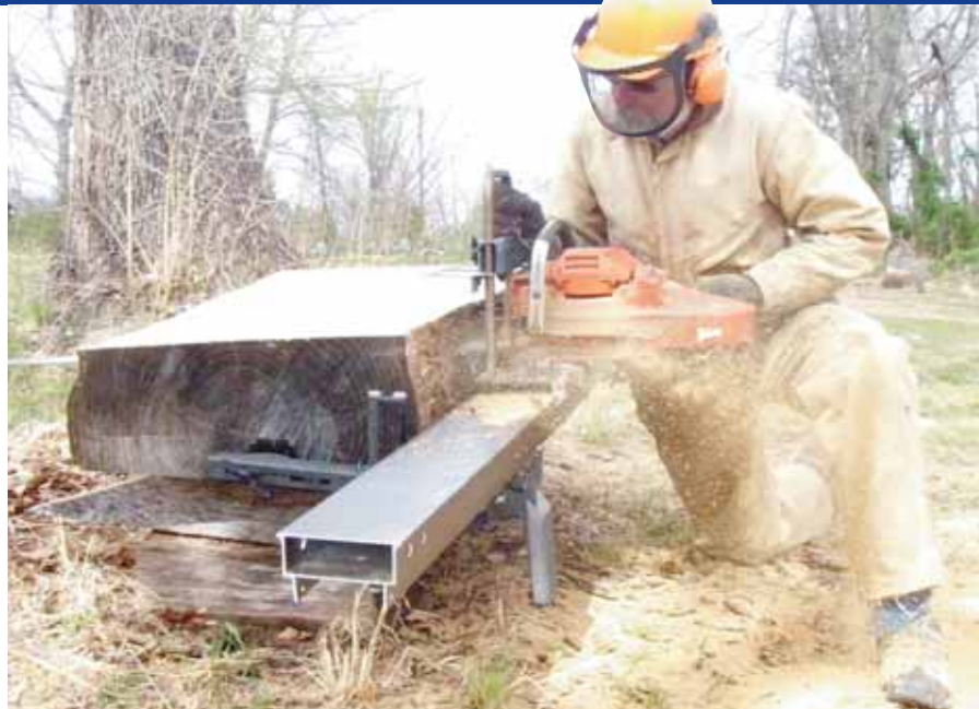
Two advantages of the guide rail system are that one person can easily use the mill, and that the bar does not need to reach all the way through the log. A sharp chain is critical for any chain saw milling.
