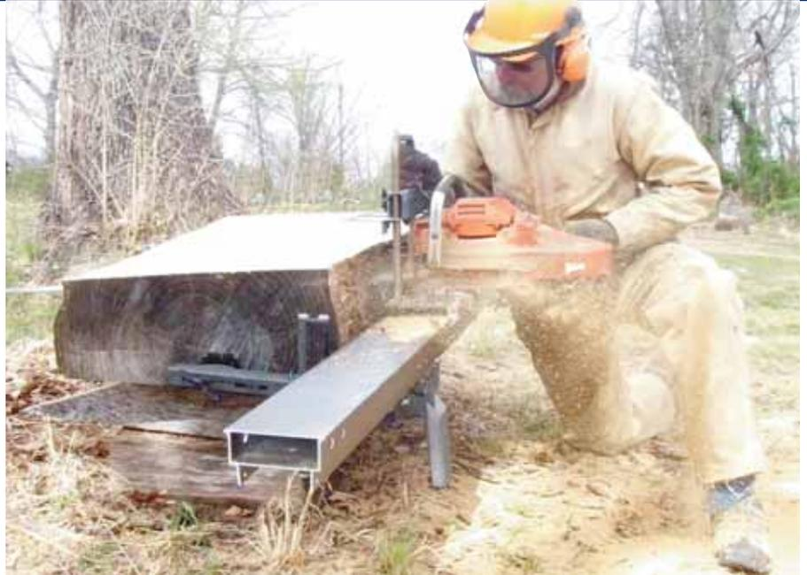
Two advantages of the guide rail system are that one person can easily use the mill, and that the bar does not need to reach all the way through the log. A sharp chain is critical for any chain saw milling.
