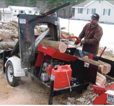
Logs do not have to be cut into shorter lengths before being pulled in by the cable (left). The blocks are cut while the log is still on the slope of the feed tray. To accommodate for this, the chain saw head is tipped at an angle to align with the log (above).
