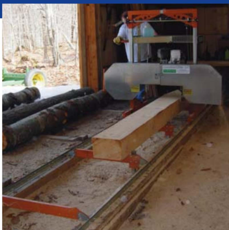
Buster Jones has added a 4-foot extension to the bed for sawing longer logs. The mill sits at ground level for easy log loading.
