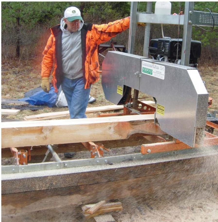
John Hricik's mill. Note that it is set on an elevation rather than on the ground.
