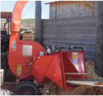
The feed chute on the hydraulic-feed model has a smaller opening leading to the two powered feed rollers.
