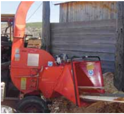
The feed chute on the hydraulic-feed model has a smaller opening leading to the two powered feed rollers.
