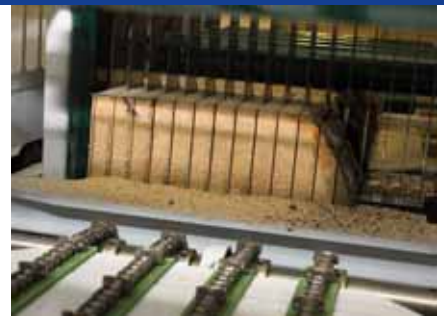
The secret behind the capacity of the Laks sawmill is a frame with up to 20 blades sawing one or two cants.
