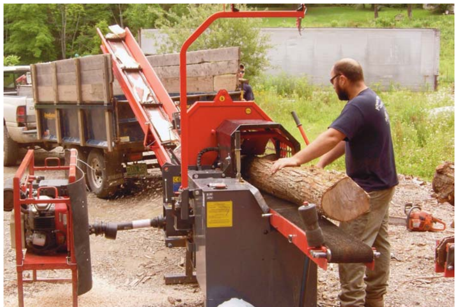
John Trombley powers his processor with a 24-hp Wood Beaver Power Pac.
