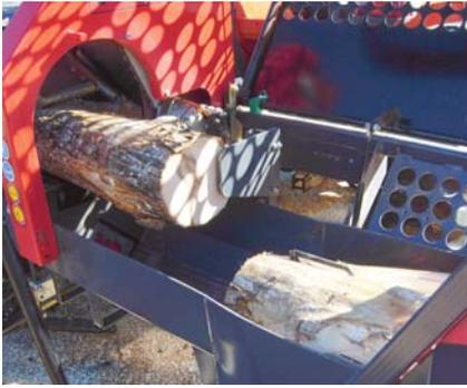
Once the block has been sawn through by the chain saw there is nothing to prevent a free fall into the cutting trough.
