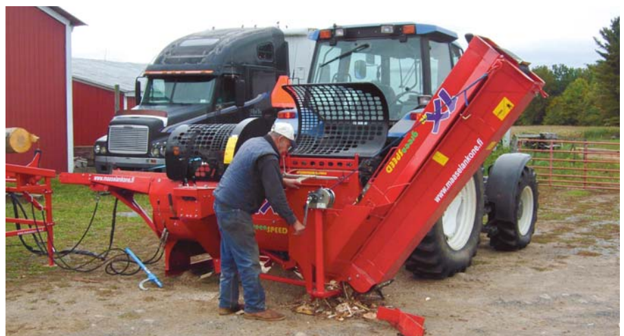
Processor in transport position on the tractor. The height is about 8 feet.
