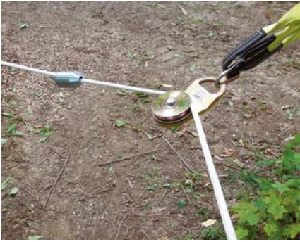
The open snatch-block with the ferrule about to reach it and pop the line out and change the direction of pull.
