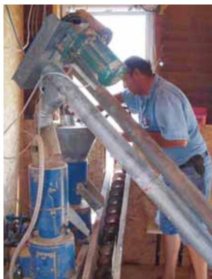
Mark adjusts a steam humidifier to get the desired moisture in the wood. His two pellet mills run off the PTO shaft (lower left in the photo) of his 150-hp Deutz tractor. The two angled pipes transfer the wood flour from the hopper to the pellet mills and the open auger transfers the pellets to a grain cleaner to remove the dust.
