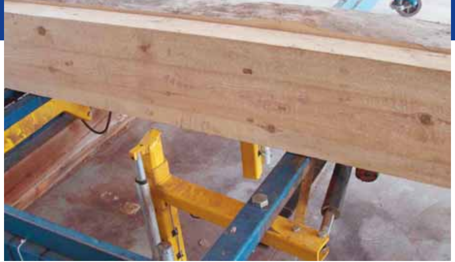
The MSG sawmill uses 12V electric motors for the clamping system. One linear actuator adjusts the clamp height, and a second one pivots the clamp into the wood.
