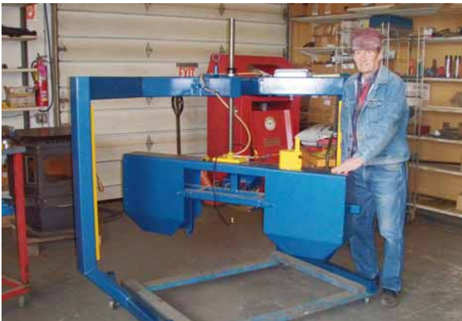
Wayne Meredith demonstrates the pivoting action of a partially built MSG sawmill. The saw is suspended from a 1-1/4-inch threaded rod, and can pivot 360 degrees.
