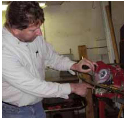
Mark Meredith demonstrates MSG's blade sharpener. Based on a chain saw sharpener, it can sharpen any pitch chain without the use of cams or adaptors.
