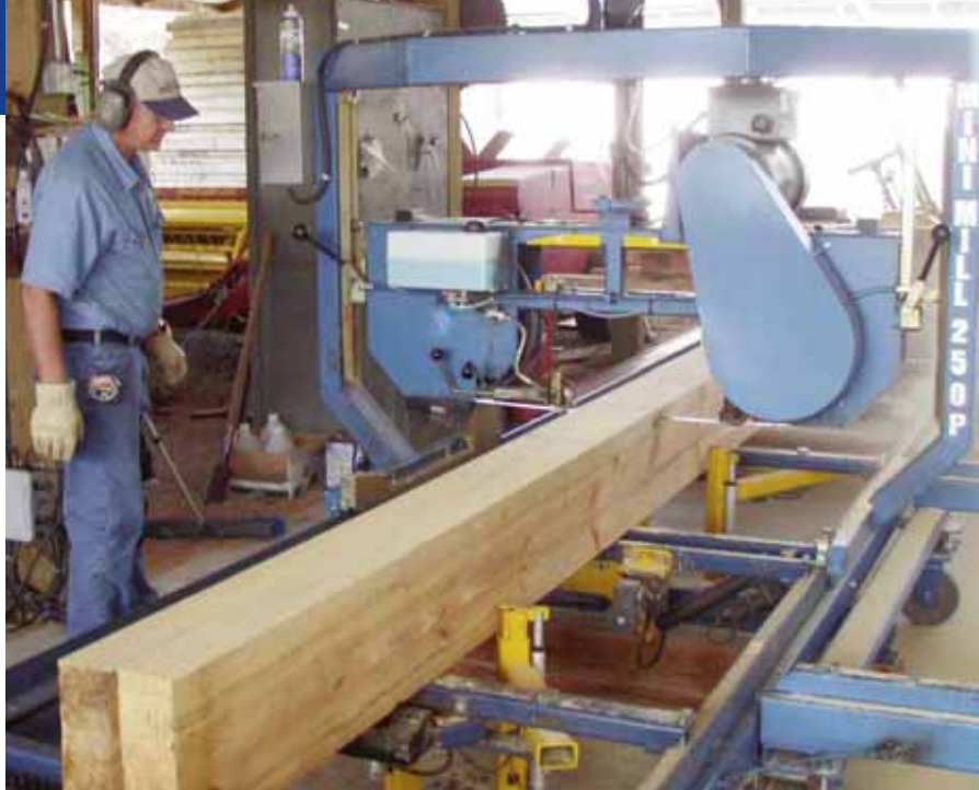
Steve Funk keeps an eye on the mill as it makes a cut. The variable-speed feed motor drives wheels on the track without a chain or cable.
