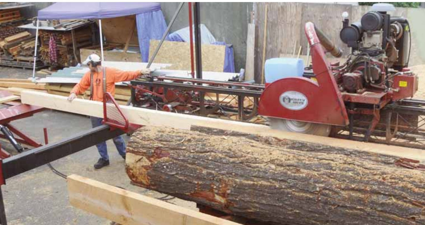
The Mighty Mite in action. The vertical main blade and horizontal edger blade produce an edged board after each pass. The drag-back brings the board back past the sawyer. According to Joolz Moorcroft, the mill works most efficiently with one or two helpers.
