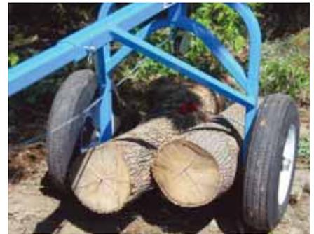
The narrow arch limited the load size when towing with a machine.
