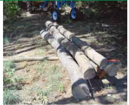
Placing a small log on the ground before bunching the logs makes it easier to choke the load.
