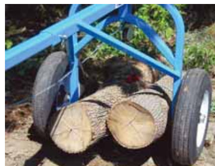
The narrow arch limited the load size when towing with a machine.
