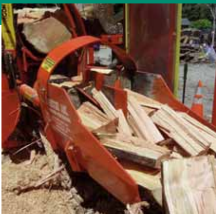
Splitter cycle time is 6 seconds and swapping splitter heads takes about 15 minutes.
