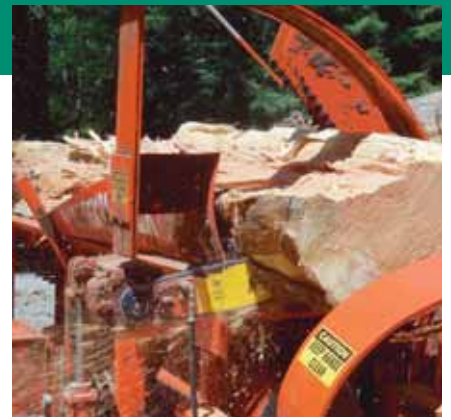
If the harvester bar chain gets dull, it can be removed for sharpening or replacement in about five minutes.
