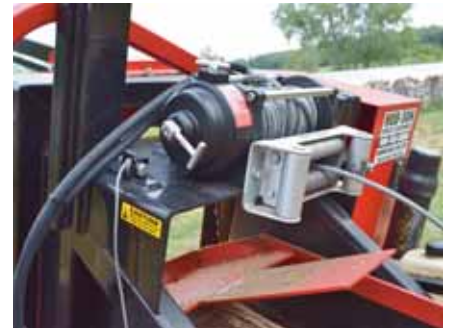
The hydraulic winch is plenty strong for loading even the largest logs.
