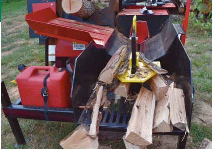
The Badger features a manually adjustable 4-way splitter head.
