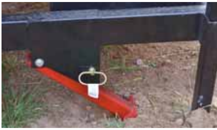
The grab-legs hold the machine while winching logs.
