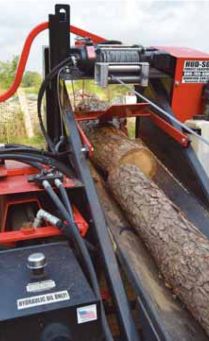
The hold-down keeps the log from sliding backwards and keeps it stabilized during cutting.
