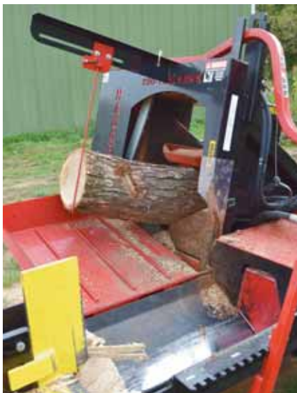
Firewood length is set by the adjustable rod.
