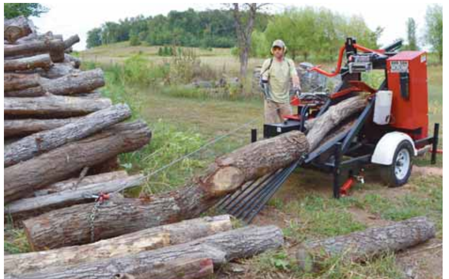
Pulling a large log into Badger’s log trough is quick and easy with the winch and choker system.
