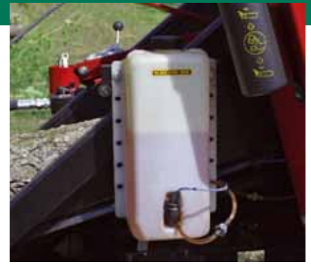
Chain lubrication is handled by the onboard oiling system that only turns on during cutting.
