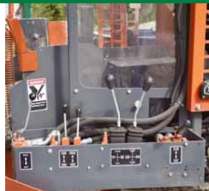
The hydraulic controls are well arranged and shielded behind Plexiglass.
