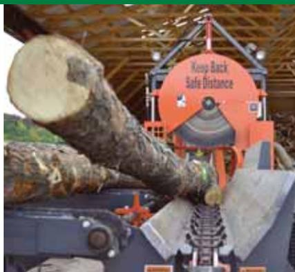
Extremely crooked logs can be a challenge for the log trough and should be cut down to shorter lengths.
