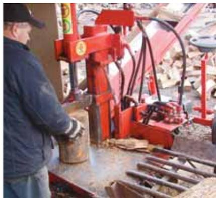
Bruce uses a shop-built hydraulic tilting feed table to keep a steady supply of wood at his fingertips. The Timberdevil's hydraulic splitting ram is activated by a simple foot pedal.
