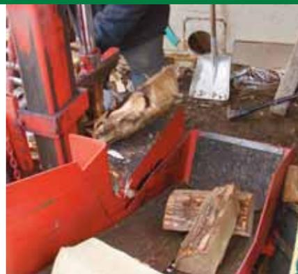
Split pieces are directed onto the attached hydraulic conveyor, providing the flexibility to load directly onto a truck, or piled on the ground.
