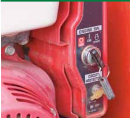
The 11hp Honda GX340 that powers Bruce's Timberdevil comes equipped with a keyed electric start, as well as a recoil backup.
