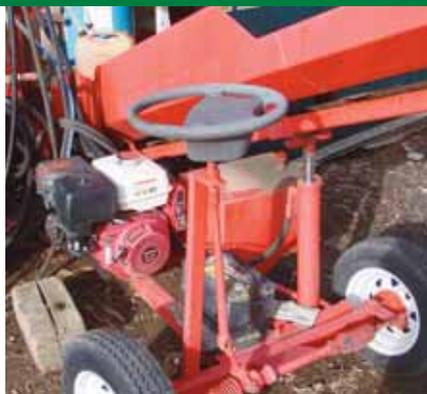
Self-propelled and equipped with an automotive-style steering wheel, the Timberdevil can be moved to the wood.
