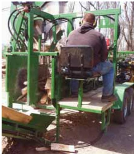
**With a consistent supply of logs, the machine can produce up to 40 cords of firewood in an 8-hour shift. The 91-hp diesel engine and variable displacement hydraulic pumps are the keys to its productivity. The 8-way splitter adjusts for different log diameters. In the three months they have run the machine, it has processed about 300 cords of firewood.**
