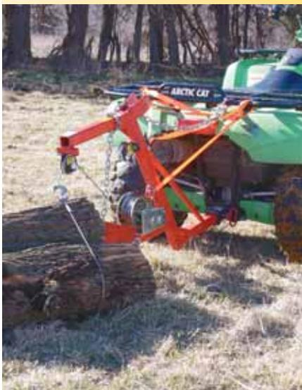
It took less than 10 minutes to hook the 90-pound log skidder to the ATV. Setting a 200-pound tank of sand on the front of the ATV was the hardest part of setting it up.
