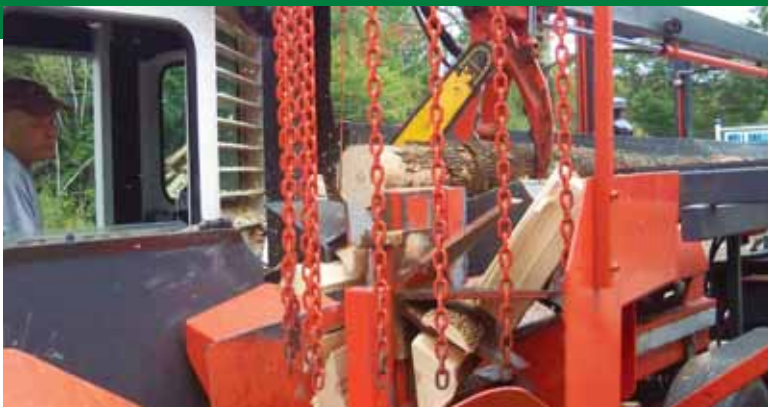
The 1/2-inch chain can handle wood up to 24 inches in diameter and the 8-way splitter head makes manageable pieces even from the largest logs. One chain cut 65 cords before having to be sharpened.
