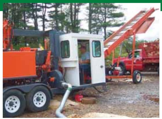
The Multitek 2040XP2 in operation. Doug shown loading a truck with green wood. Even the saw chips and splinters get used.
