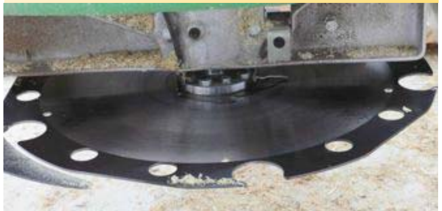
The 25-in. blade on the Lucas 10-30 can mill up to a 10-in. by 10-in. timber in one pass.
