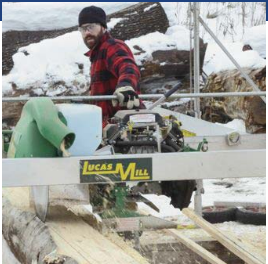
With its Kohler 30 hp EFI engine, the 10-30 had no issues powering through whatever was put in front of it.
