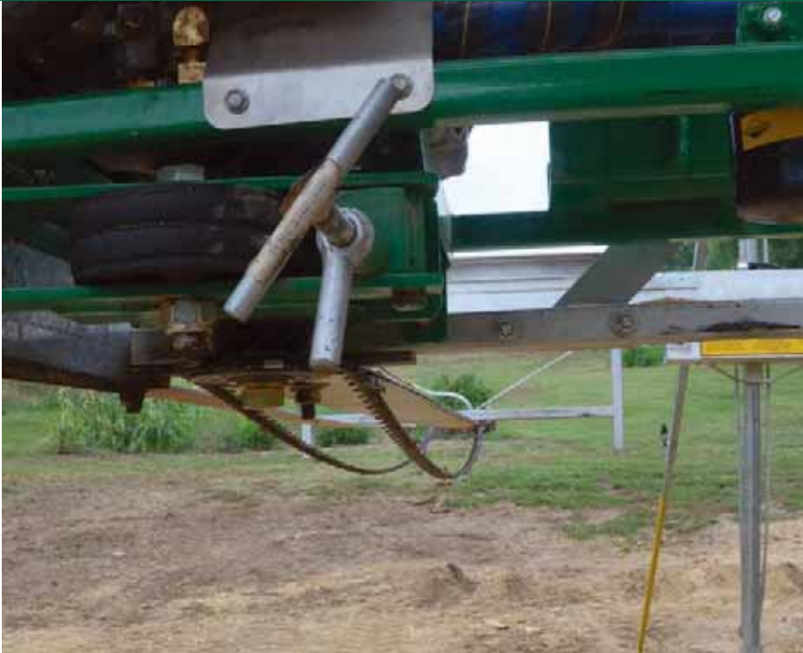
With ample adjustment in the tensioning mechanism, swapping chains can be accomplished in a couple of minutes.
