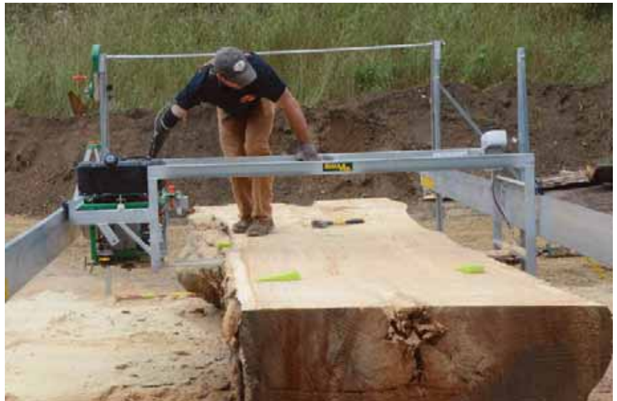
Above: A hammer and wedges kept the slabs from pinching as I was cutting. Below: The Lucas DSM23 deep throat slabber powers its way through over 60 in. of wet, stringy cottonwood.
