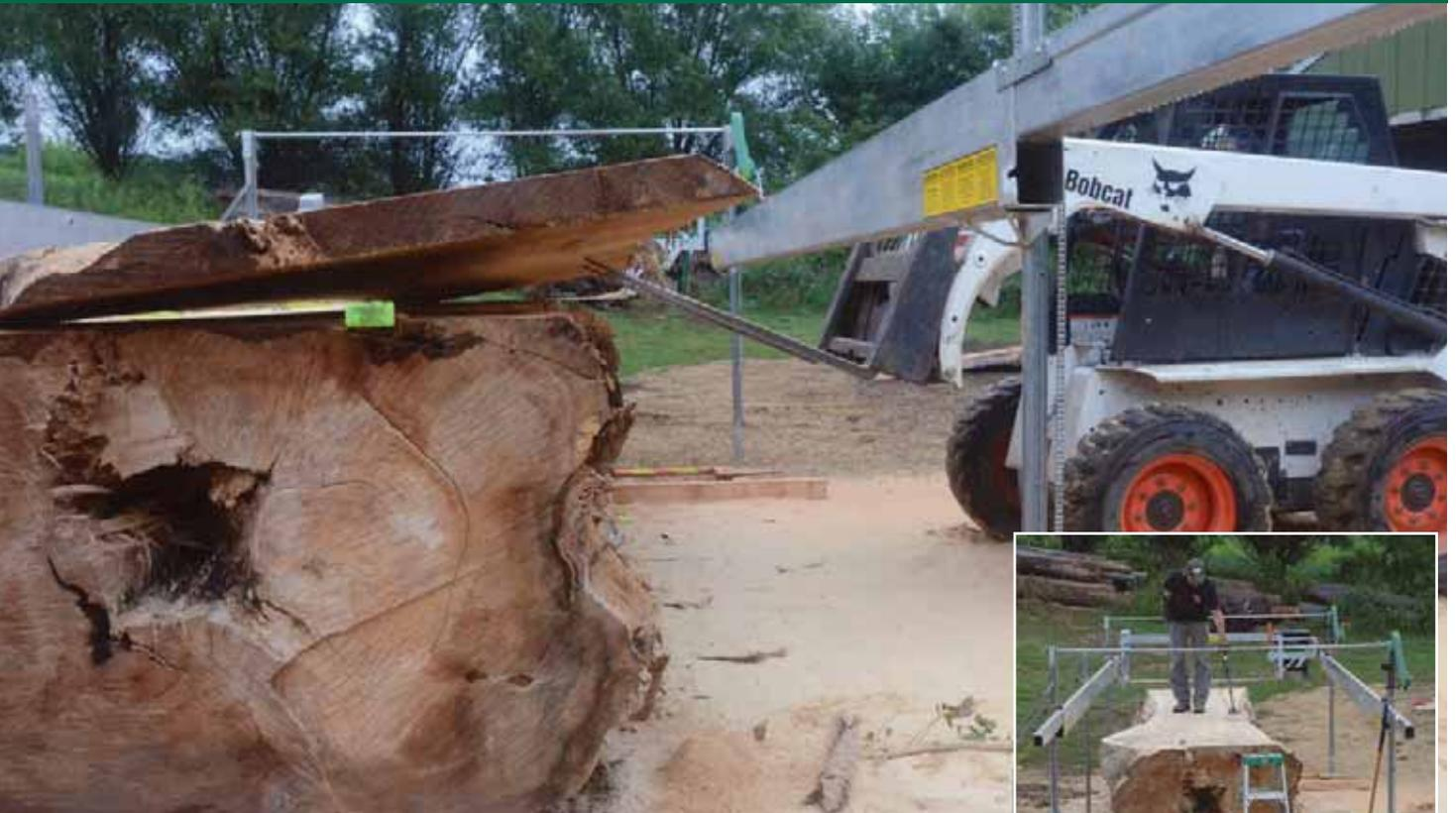
A piece of equipment to move the slabs is an absolute must when it comes to slabbing large logs.
