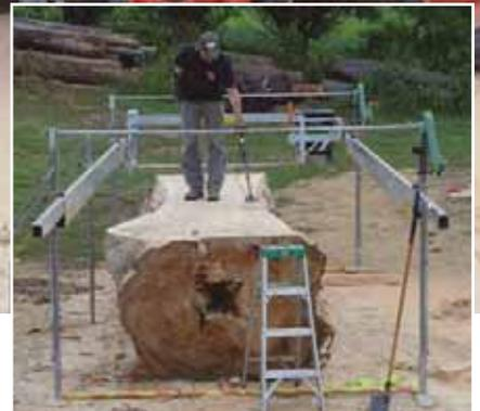
The log was scanned after every slab and, despite being a yard tree, was surprisingly without metal.
