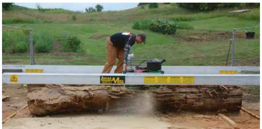
Above: A hammer and wedges kept the slabs from pinching as I was cutting. Below: The Lucas DSM23 deep throat slabber powers its way through over 60 in. of wet, stringy cottonwood.
