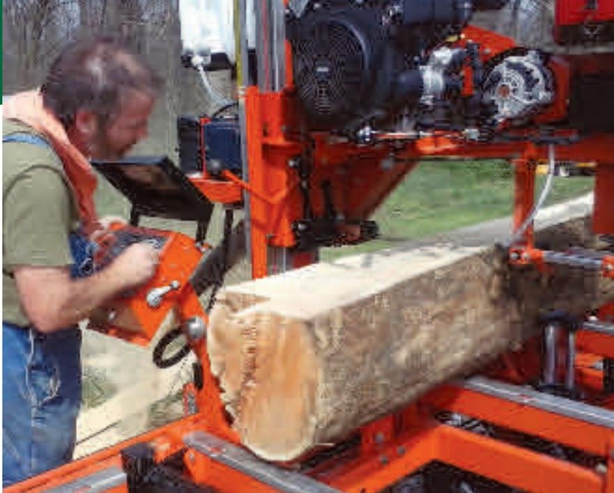
Wakefield keeps an eye on the cut and listens for changes in the motor as he keeps a hand on the electronic feed speed control. The speed control is smooth and precise, and automatically stops the carriage if it encounters resistance.
