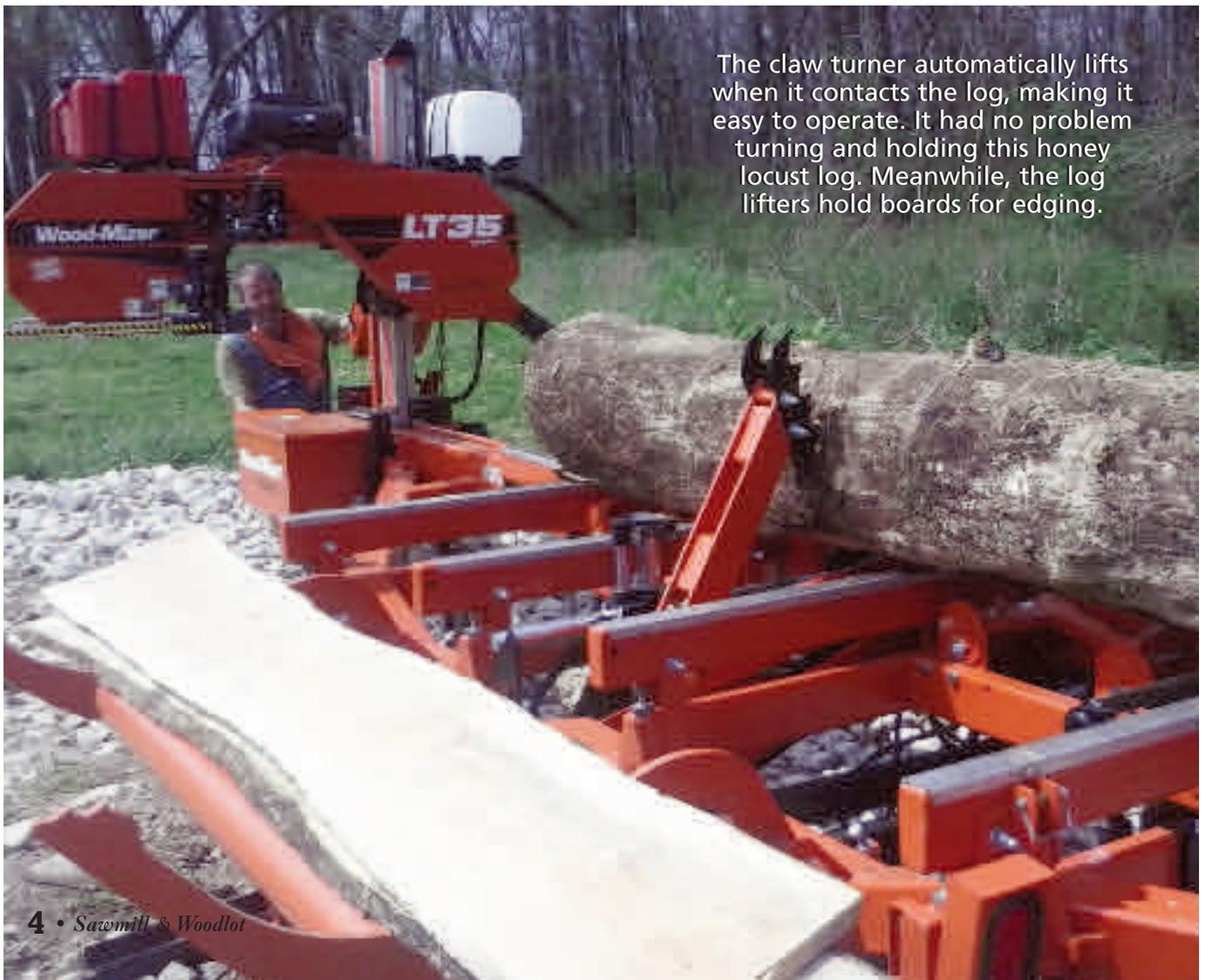
The claw turner automatically lifts when it contacts the log, making it easy to operate. It had no problem turning and holding this honey locust log. Meanwhile, the log lifters hold boards for edging.
