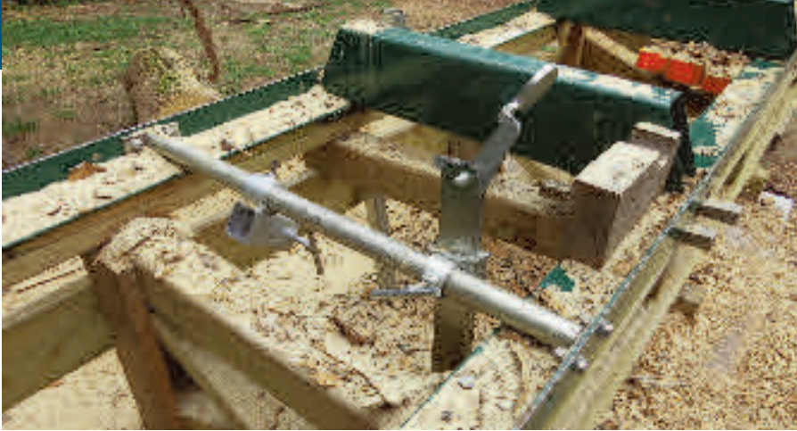
The cam-locking log dogs are quickly and easily adjusted, and maintain a secure hold on the log while milling.
