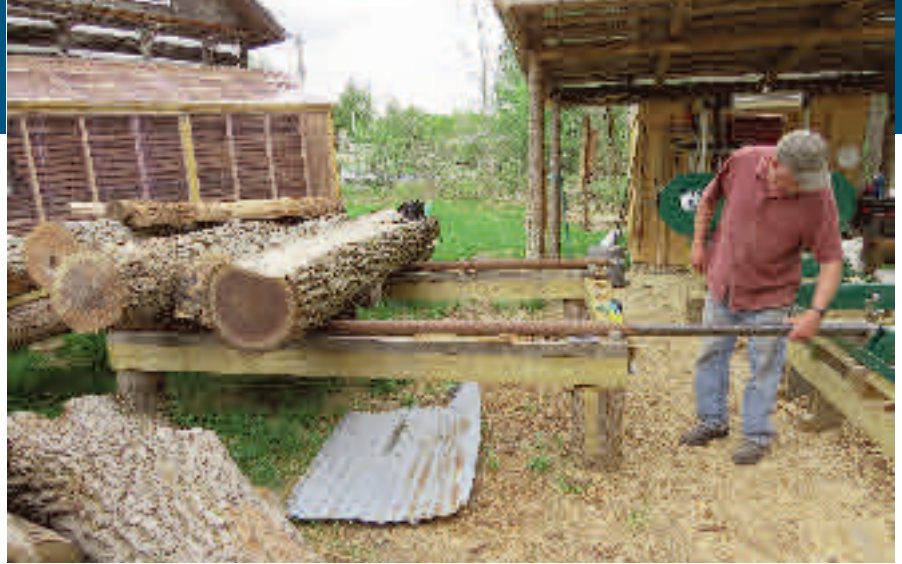
Michael slides the telescoping log supports from the log deck before rolling the next log onto to the mill. When extended, the pipe section rests securely in a contoured block of hardwood secured to the mill deck. His recently constructed solar kiln, with a full load of black walnut lumber, is visible behind.
