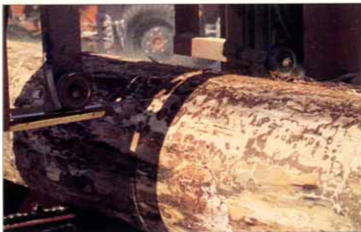
TimberKing designed the B-20 to run a 1 1/4-inch wide bandsaw blade with offset teeth and a kerf of approximately 0.080 inch.
