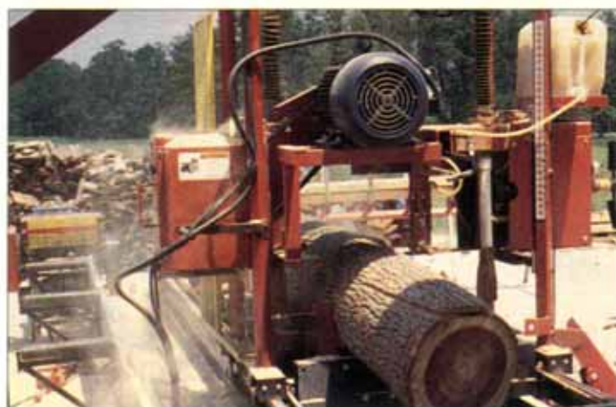
With good help and a long day of sawing, J Brady says he can cut 1,000 board feet of lumber with his B-20.
