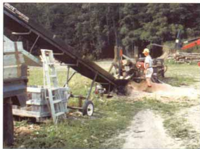
Dave Hannum uses a conveyor to load wood from his processor onto a truck for delivery.
