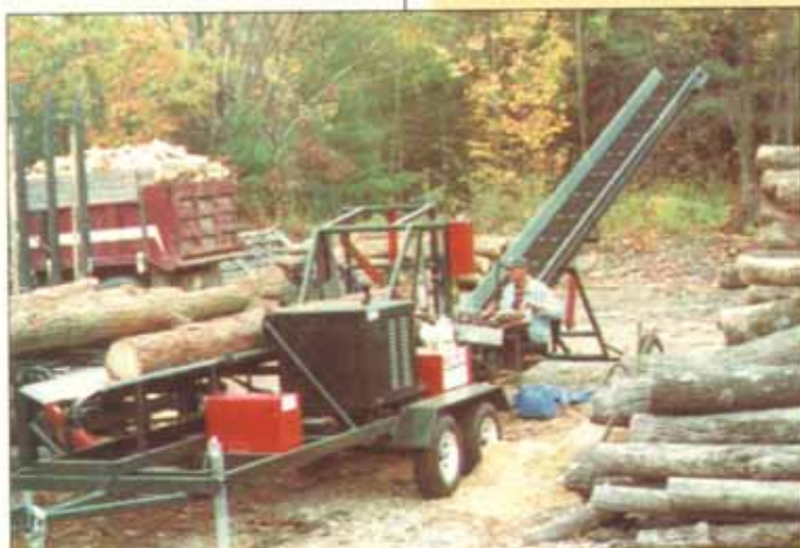
The Wilbur brothers added a conveyor to speed their operation.
