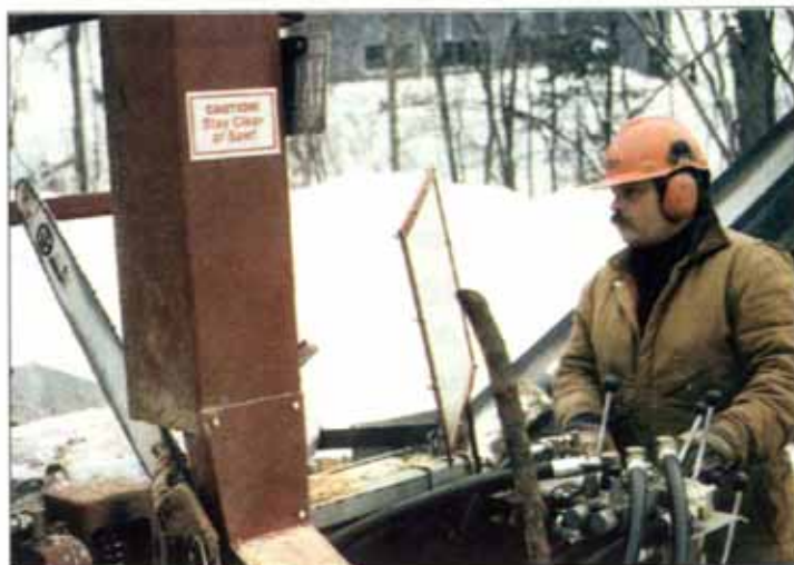
Bret Lewis stands at the controls. He is in safe location, note the protective viewing shield.
