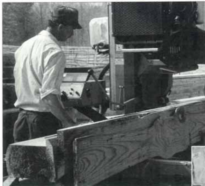
Duke demonstrates how he uses the sawmill itself as an edger by lining up boards alongside the cant he is sawing. With a little prior planning, this method can save a sawyer time. Inset: Wood-Mizer offers a debarker on the LT40 Super, something Duke says extends his blade life considerably.
