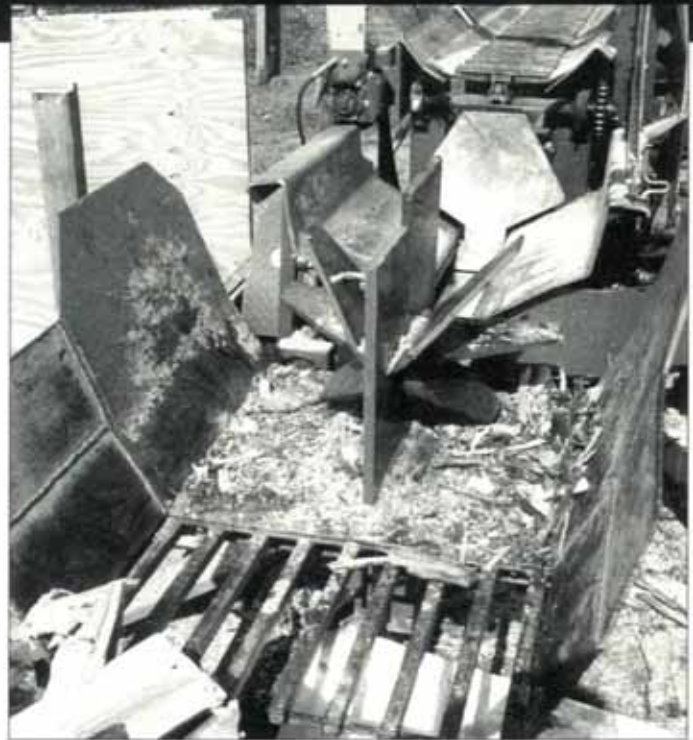
Bill Rowe installed a tongued grate forward of the splitting head to remove fines from his firewood. A conveyor salvaged from a grain elevator carries the waste that drops through the grate away from the machine.
