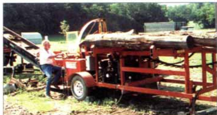
The B-2 comes with an operator's seat as standard equipment, something Bill Rowe finds useful. Rowe and other users have said the B-2 could use a longer log deck.
