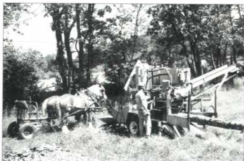
Bruce Cheney's Chomper is an ideal workmate with his team of Belgians. Because the machine is at ground level, the logs can be dropped by the horses within easy reach of the winch cable.
