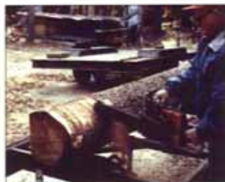
Larry's mill is hand-dogged and he uses a chainsaw debarker to clean his logs.
