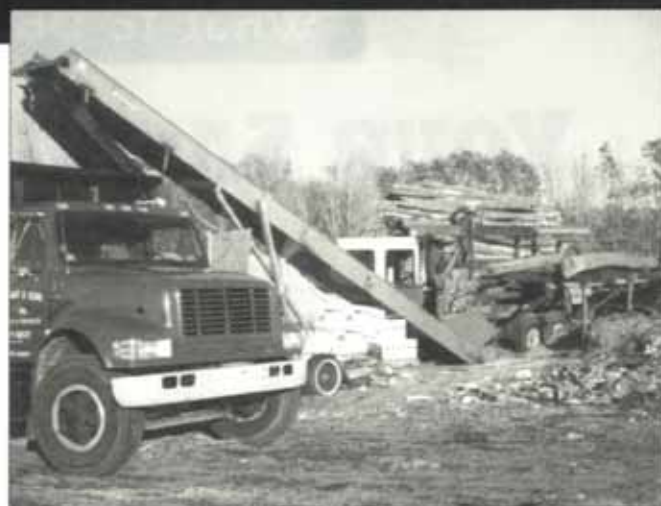
Richard Smart's deflector chute can be seen at the top of his conveyor in this photo.
